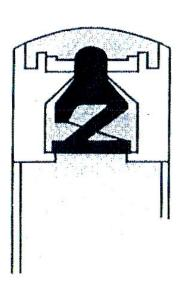
The Accu-Dyne Test Marker Pen has a special spring loaded valve applicator which seal off the Dyne Fluid in the pen barrel thus preventing contamination and evaporation.
