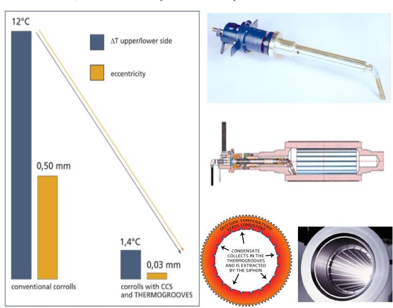
The university of Coburg has made a test run with a conventional system and our CCS/Thermogrooves. The figures in the diagram show the temperature difference of the top and bottom of the corrolls as well as the distortion after a stop of 30 minutes
